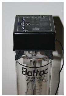
Boltac Industries SSVI-3 (Stirred Sludge Volume Index Stirrer v3) unit is designed to meet/accommodate Standard Methods requirements.
